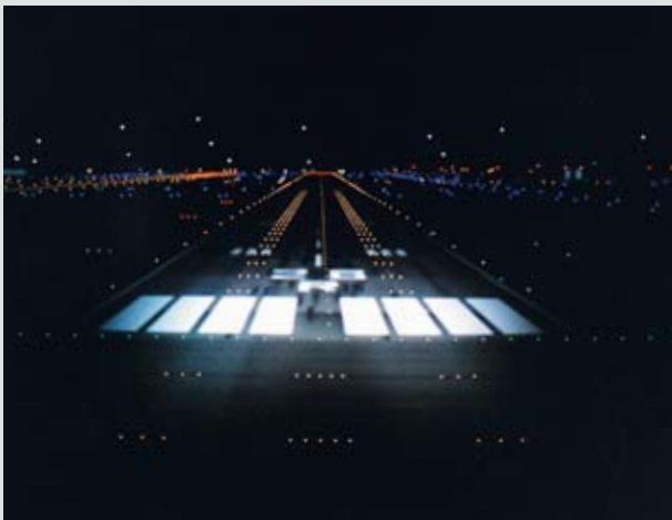
Calligraphic light points on a simulated runway. Photo courtesy CAE Electronics Ltd., Montreal, Canada.
