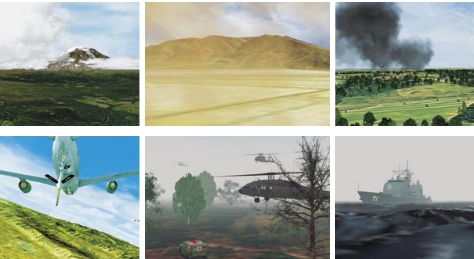
FlightSafety's state-of-the-art VITAL X visual system uses a multi-channel, Liquid Crystal on Silicon (LCOS) projector to display the MCTT's high-resolution, photo-realistic images. VITAL X employs the Beaufort scale to classify three-dimensional sea states, simulating realistic calm and light seas, strong gales, and changes in wind speed and direction.
