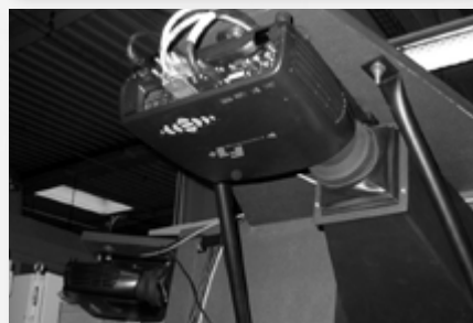
Photos: The Royal Dutch Army uses hundreds of projectiondesign projectors in their TACTIS (Tactical Indoor Simulator), in which personnel is trained on the Leopard 2A6 combat vehicle.
